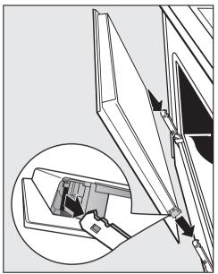
Hold the door securely at both sides and carefully fit it back into the hinge retainers. Open the door fully.
